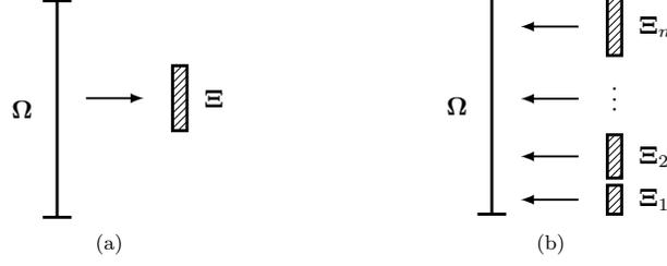
Figure 7. Projection between cell face and mortar: (a) from a left face to the left side of a mortar, (b) from mortars back to the left face.
