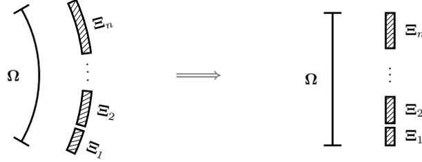
**Figure 6.** Mapping of curved cell face and mortars to straight ones: left, curved face and mortars in physical domain; right, straight face and mortars in computational domain.
