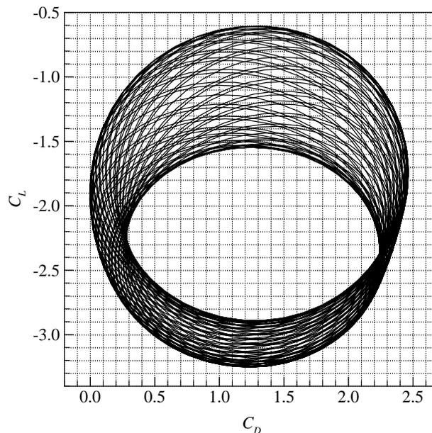
Figure 27. Lissajous curve of  $C_L$  and  $C_D$  in 20 rotating periods (from  $tU_\infty/D = 120$  to 200) for a rotating triangular cylinder.
