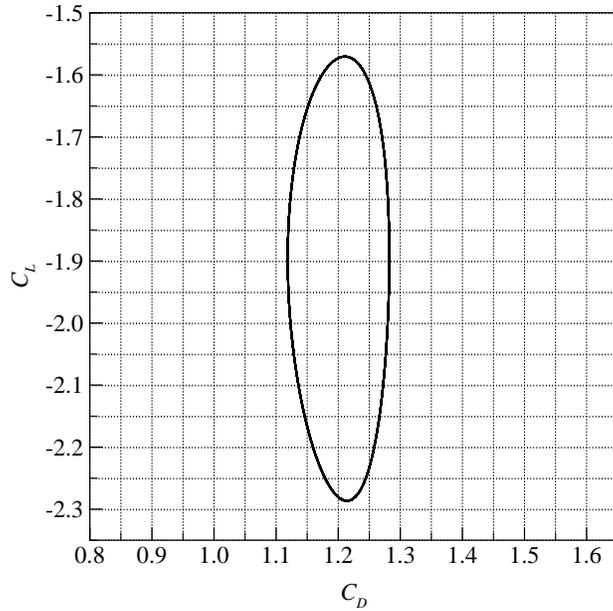
Figure 15. Lissajous curve of  $C_L$  and  $C_D$  in 20 rotating periods (from  $tU_\infty/D = 120$  to 200) for a rotating circular cylinder.
