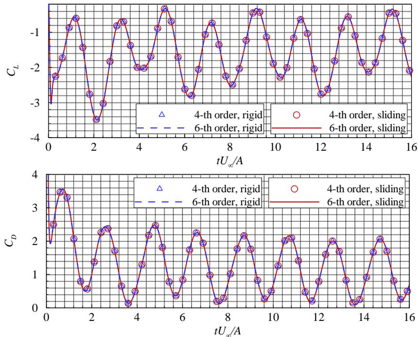
Figure 19. Comparison of transient lift and drag coefficients for a rotating elliptic cylinder from the 4-th and the 6-th order schemes on a rigid-rotating mesh and a sliding mesh.
