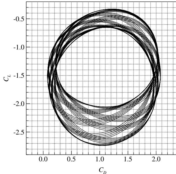
Figure 21. Lissajous curve of  $C_L$  and  $C_D$  in 20 rotating periods (from  $tU_\infty/D = 120$  to 200) for a rotating elliptic cylinder.
