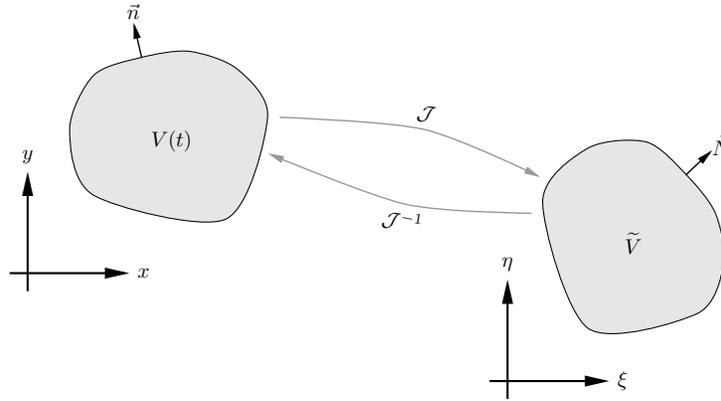
Figure 1. Mapping between a moving physical domain and a fixed computational domain.
