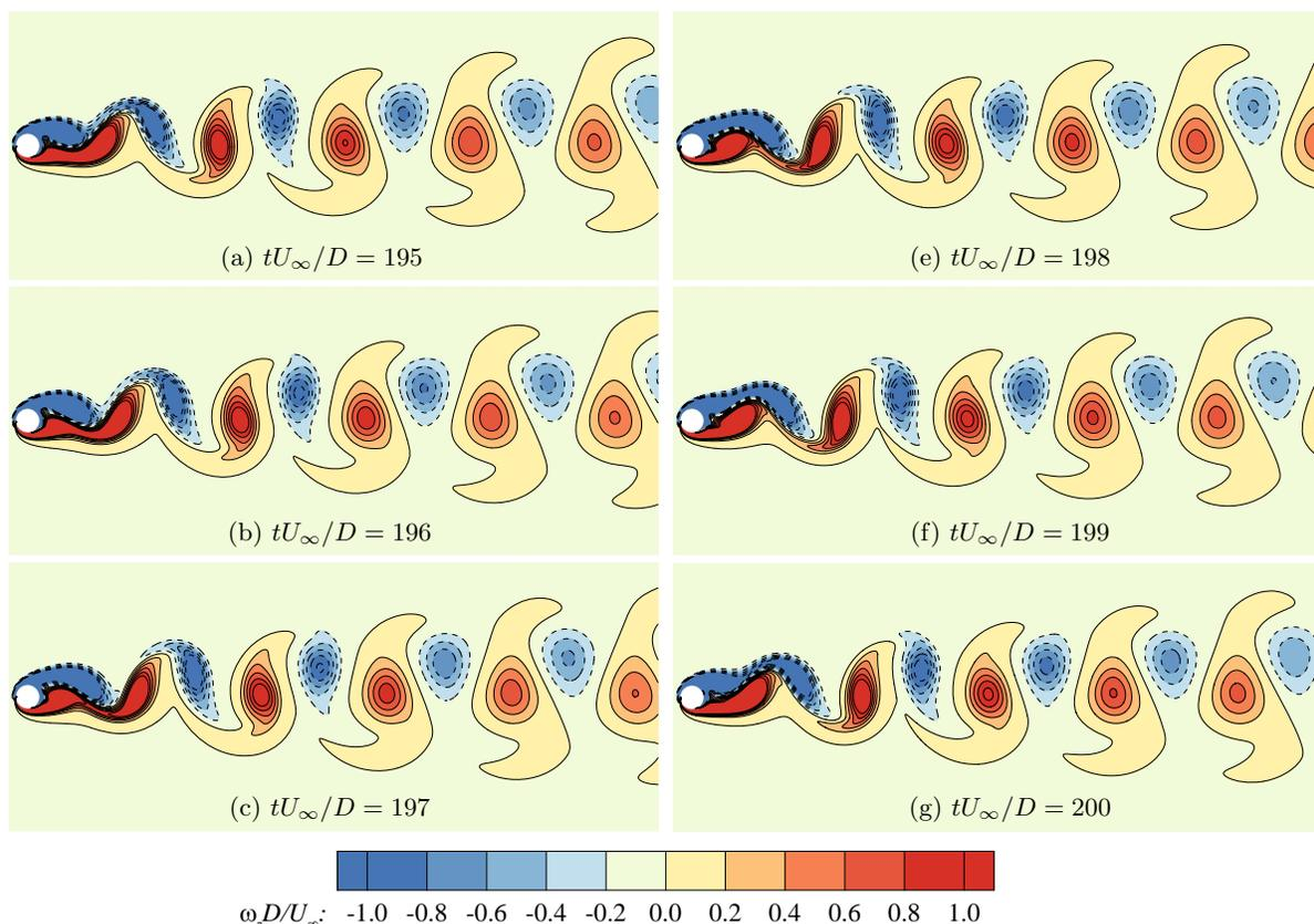
Figure 17. Comparison of vorticity contours from sliding mesh (lines) and static mesh (colors) for flow over a rotating circular cylinder.
