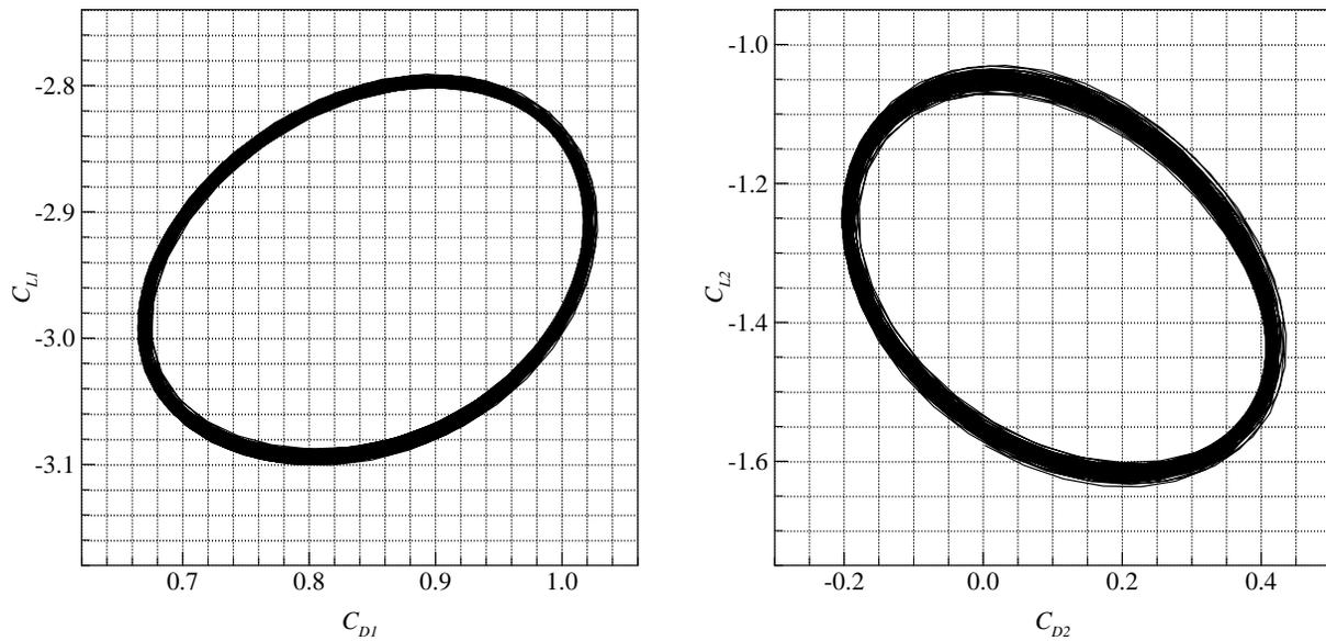
Figure 37. Lissajous curves of  $C_L$  and  $C_D$  in 20 rotating periods (from  $tU_\infty/D = 120$  to 200) for two tandem rotating square cylinders.
