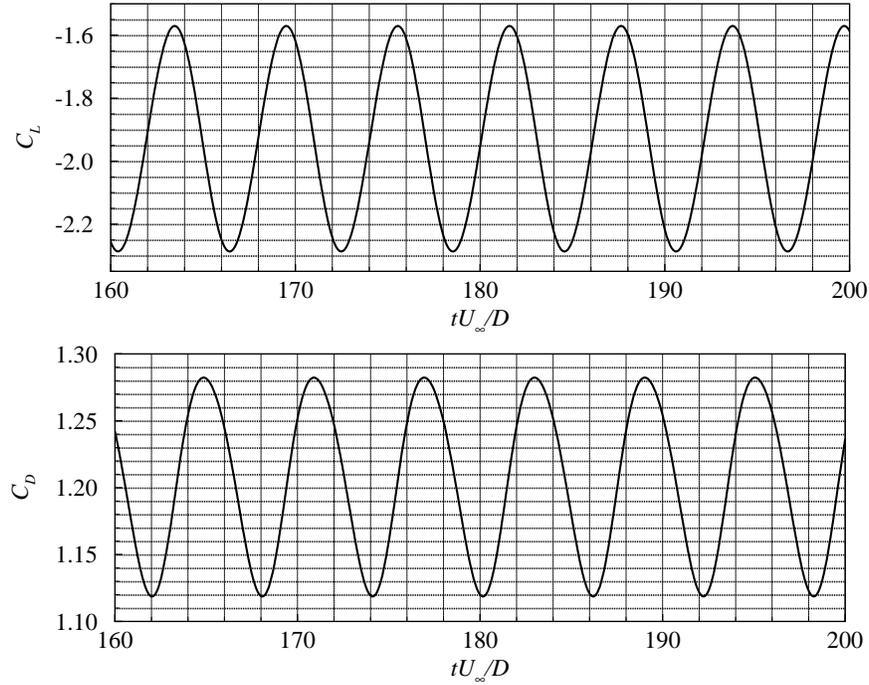
Figure 14. Converged lift and drag coefficients for flow over a rotating circular cylinder.
