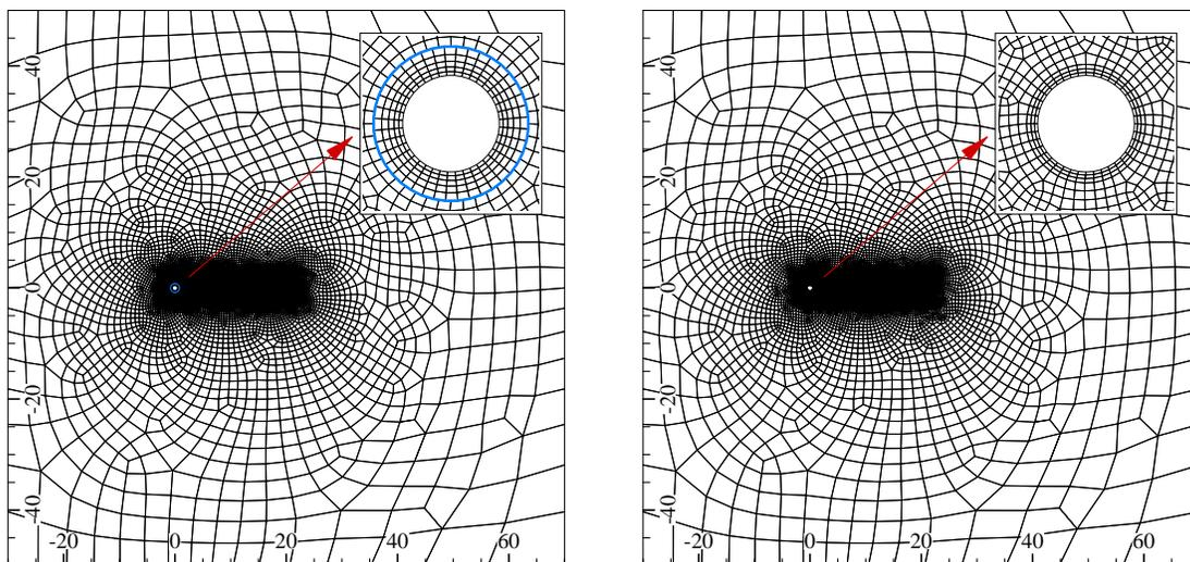
Figure 12. Global and local views of the sliding mesh (blue circle represents sliding interface) and the static mesh (right) for a rotating circular cylinder.
