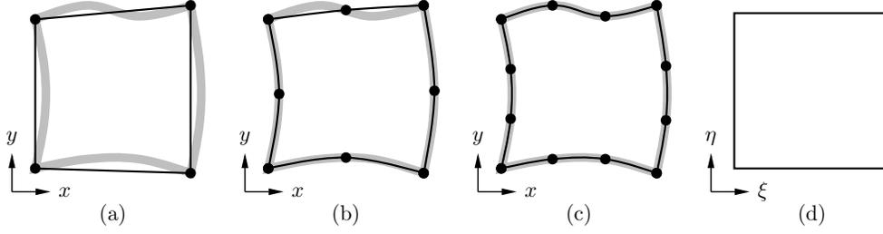
**Figure 2.** Iso-parametric representations (black lines) of a curved element (wide gray lines): (a) linear representation,  $K = 4$ , (b) quadratic representation,  $K = 8$ , (c) cubic representation,  $K = 12$ , (d) a standard computational element.
