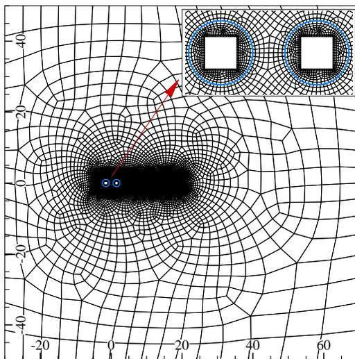
Figure 35. Mesh for two tandem rotating square cylinders (blue circles indicate sliding interfaces).
